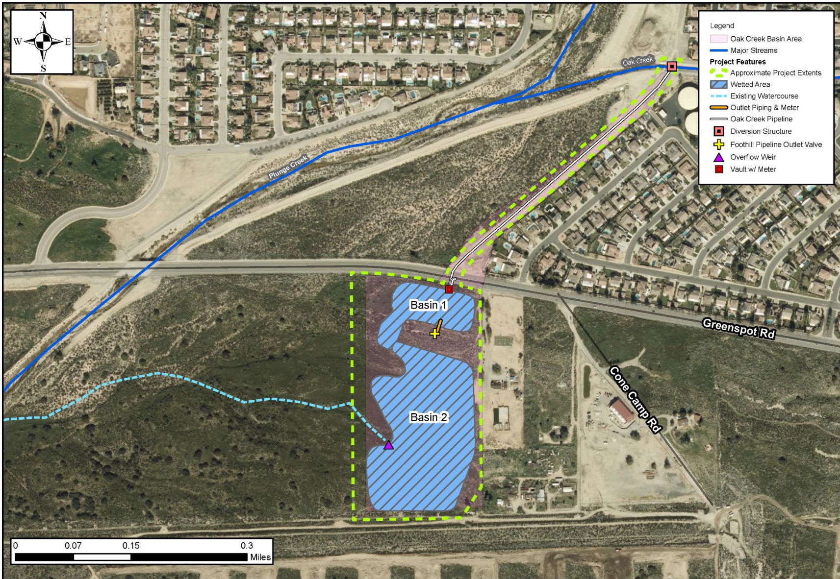
Figure 5. OCRB Construction Alternative Overview
